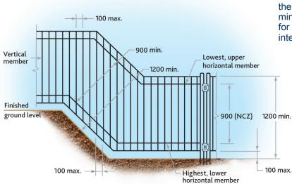
Note: On sloping sites, the fence height is to be measured perpendicular to the ground line.
