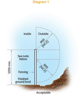
Note: The lower radius point may be anywhere on the fence at least 900mm above the ground or the highest lower rail or foothold.
