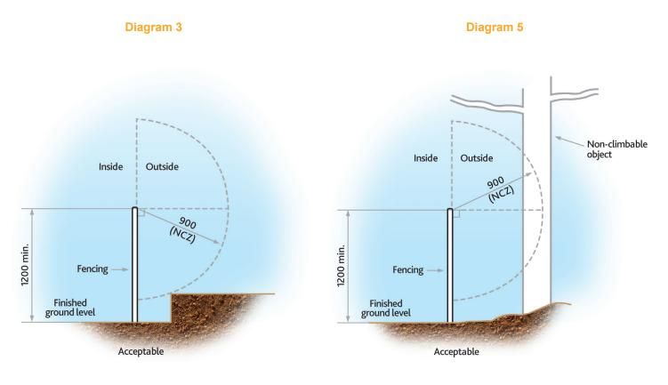
Note: The minimum height of a safety barrier is 1200mm and is measured on the outside of the barrier. The above acceptable projection must not reduce the effective height of the fence less than 1200mm.
